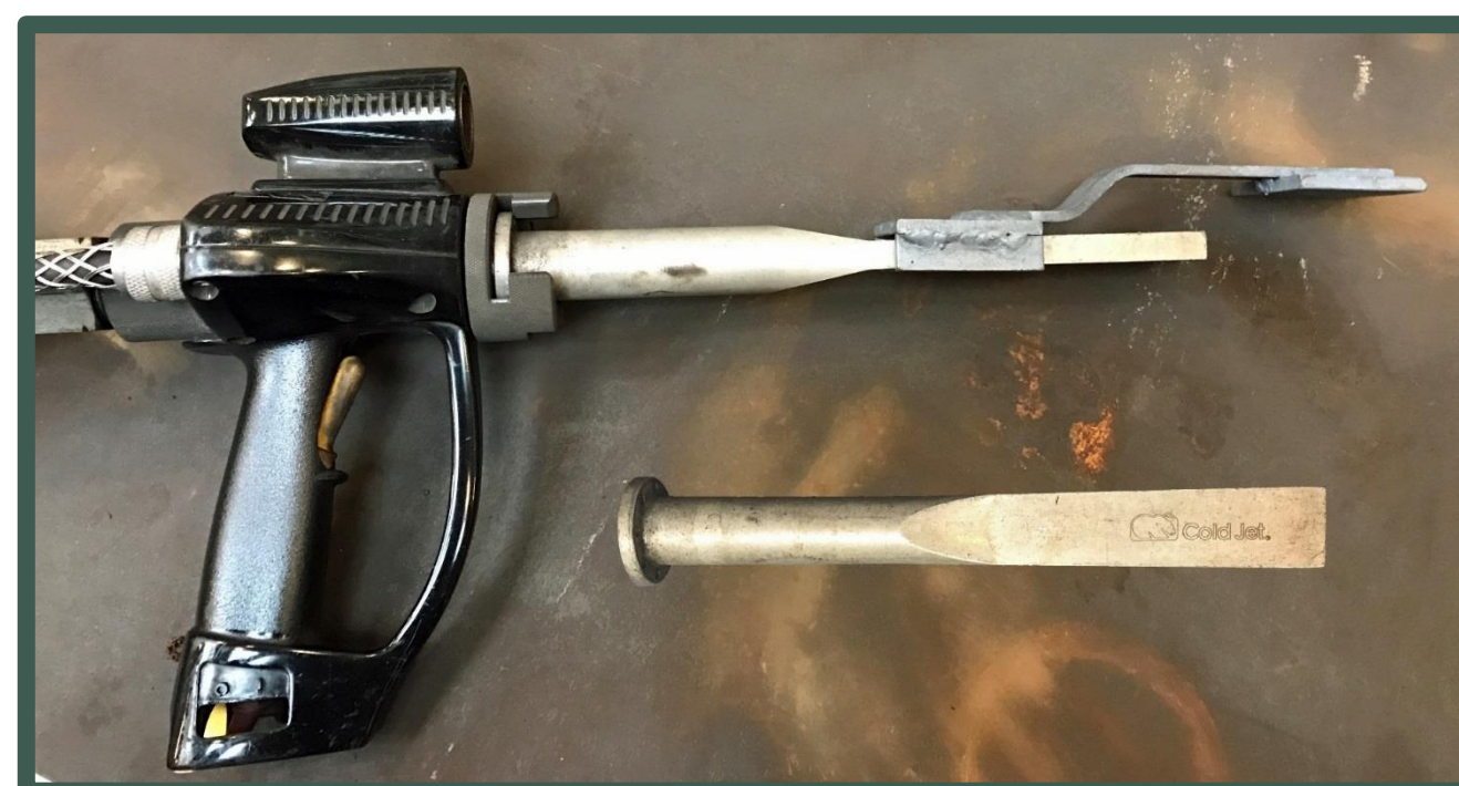
Fig 8: Unit blast nozzle with attachment to regulate distance during sample testing
