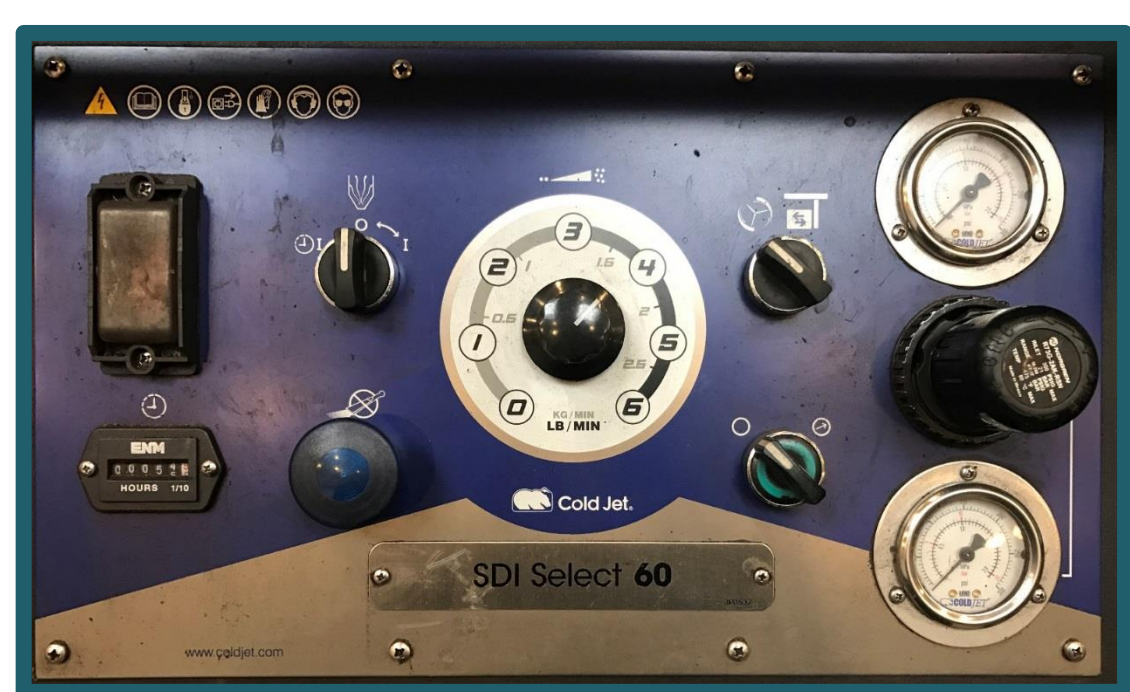
Fig 3: Detail of unit control panel. The ColdJet SDI Select 60 has a variable feed rate of 0-6 lb of aggregate per minute and a blast pressure range of 20-250 psi. The blast applicator has an interchangeable nozzle connector.
