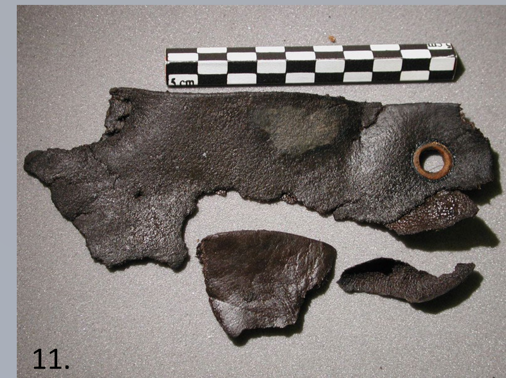
Fig. 10: Leather sample before chelating agent testing. Fig. 11: Waterlogged leather sample after diammonium citrate 5% w/w bath. Fig. 12: Leather sample after polyethylene glycol treatment and freeze drying.
