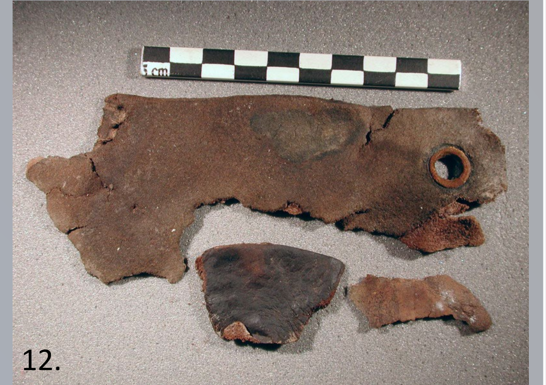
Fig. 10: Leather sample before chelating agent testing. Fig. 11: Waterlogged leather sample after diammonium citrate 5% w/w bath. Fig. 12: Leather sample after polyethylene glycol treatment and freeze drying.
