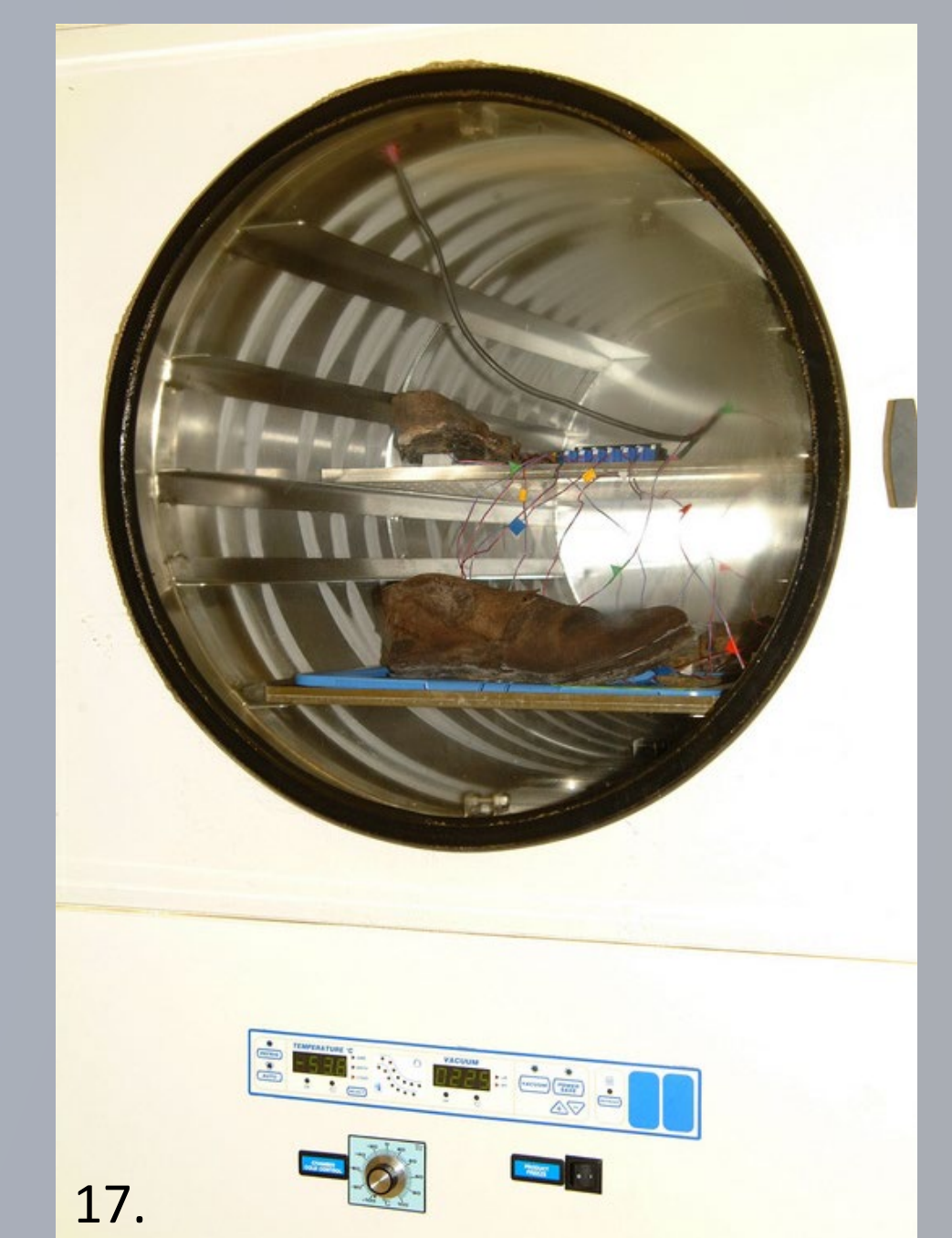
Fig. 13: HL-1501 before cleaning. Fig. 14: HL-1501 during mechanical cleaning. Fig. 15: HL-1501 after chemical cleaning. Fig. 16: HL-1501 After freeze drying. Picture taken in 2004. Fig. 17: HL-1501 during freeze drying.
