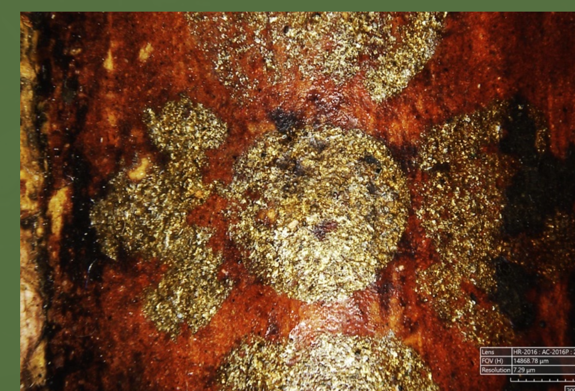
Photomicrograph of Altar Table showing brass particles (rag rdul) used for decoration, 20x magnification
