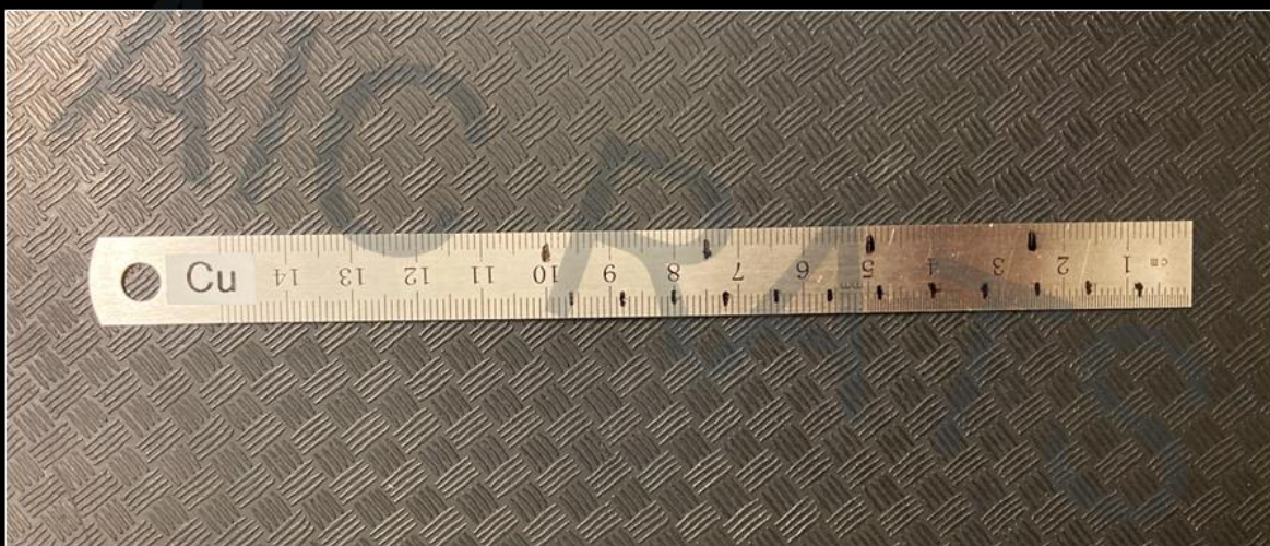
Ruler for cutting Cu coupons, marked at 2.5 cm (coupon length) and 0.8 cm (coupon width) increments
