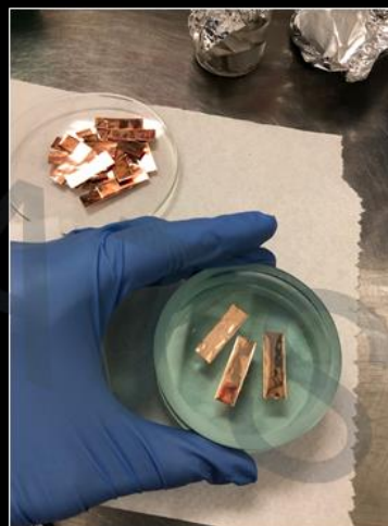
Glass canning weights (left), and their use flattening copper coupons before assembling the test (right)
